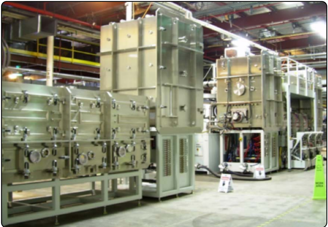
Figure 4 – Large-scale CIGS Deposition Tool Capable of Processing 1 m Wide Web to be Installed at USPVMC Manufacturing Development Facility
